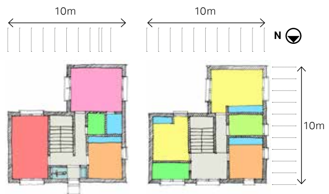
C4. L-shaped 4 bedroom house Either as a corner building or as a two-storey extension of the type B2
