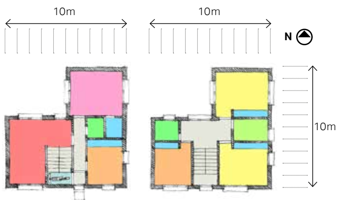
C3. L-shaped 4 bedroom house Either as a corner building or as a two-storey extension of the type B1
