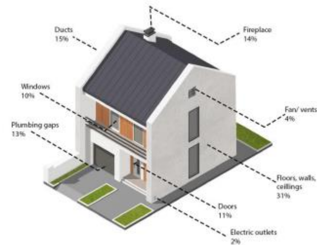
Figure 17 - Energy loss through a building
